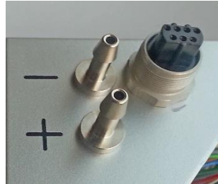
Fig. 3: Differential pressure connections and E2 socket on the underside of the device
