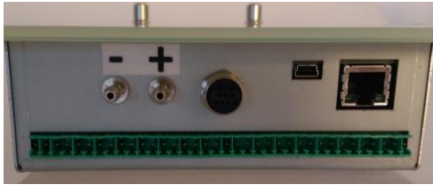
Figure 8: CRP5 connections with external HC2 probe
