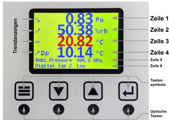
Figure 11: Operating keys and display in the CRP front panel
