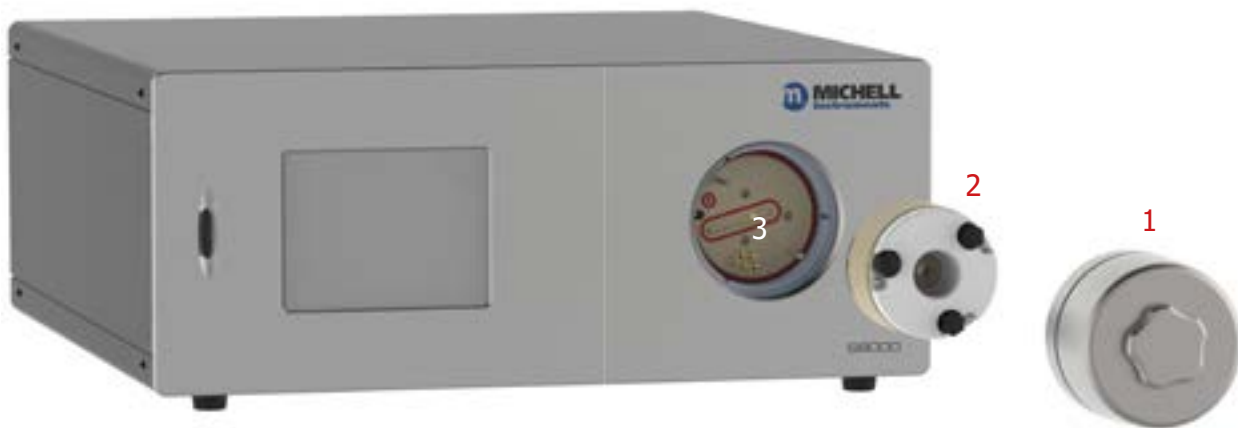
Figure 35 Sensor Mirror Cleaning
